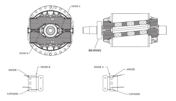
Figure 3. The 2-Pole Rotor Assembly 8/10kW
